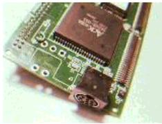
the DIN-8 pins can be desoldered. The easiest (and pretty ruthless) way is to cut slowly through the plastic of the connector, cut one of the pins, grab it with needlenose pliers, and heat up the solder joint until it comes out.
