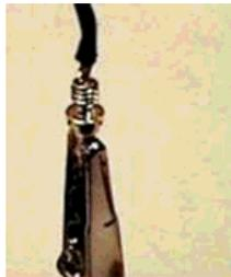
3. Insulate using the red and black duct tape. For a more solid connector, cover the solder joints with epoxy before taping. The final result should look like:
