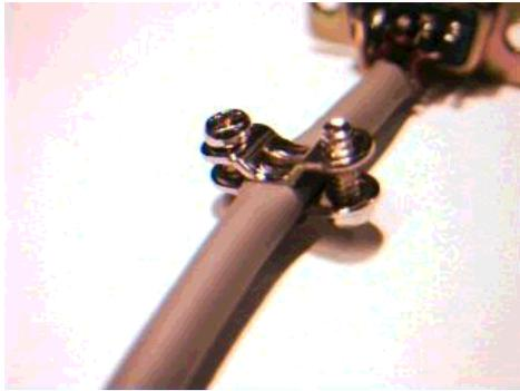
Place the assembly into the DB9 case, slide the 2 fastening screws into place, and put the 2 RS232 captive screws in their positions
