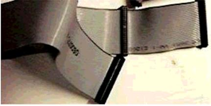
goes to the CPU board, the other to the hard drive. The cable is keyed, and the position of the connector on the cable does not matter. Power to the drive is provided through the cable.
