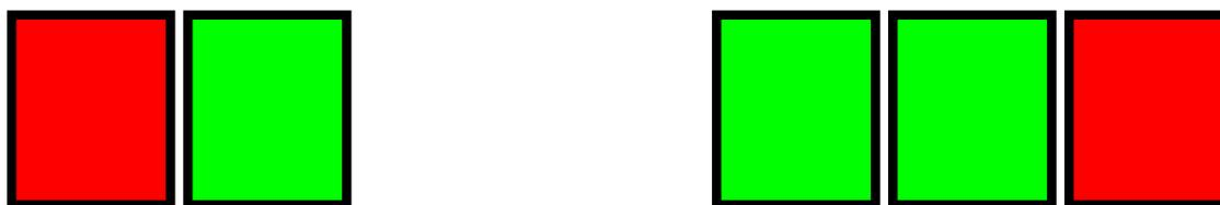
Figure 2-14: A visual tag representing the value ten. Squares at either end are red while the inner squares representing the bits are green.
