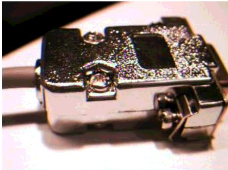
The captive screws enable fastening the Private Eye connector to the case.
