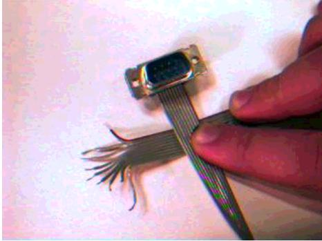
4. Solder the leads into the driver board according to the following table. Wire number 1 on most serial cables is a different color than the rest (e.g. red). Looking at the bottom of the Private Eye driver board (the side WITHOUT the large chip), the holes are numbered
