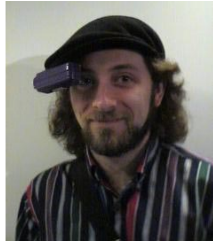
Figure 3: The Private Eye mounted on a hat’s brim.
