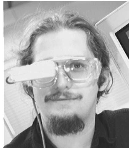
Figure 2: A safety glasses mounting of the Private Eye.
