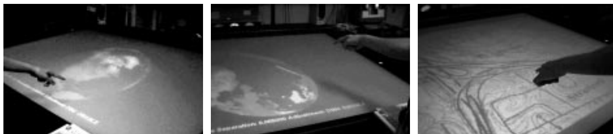
Figure 15: Terrain navigation using deictic gestures: (a) panning; (b) rotation (about an axis perpendicular to and through the end of the rotation lever); (c) zooming in.
