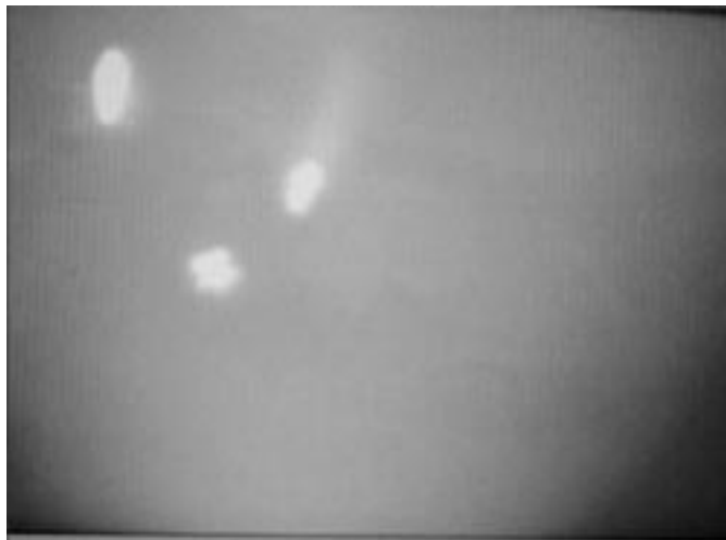
Figure 3: Image of reflection from the IR lights underneath the desk, as seen from the infrared camera.
