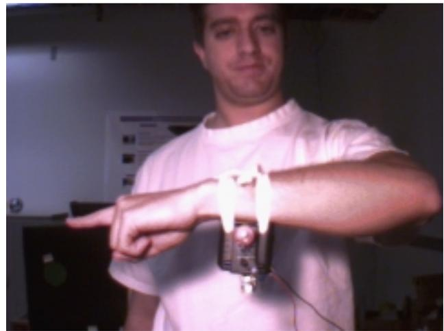
**Figure 9.** The machine used to simulate tremors
