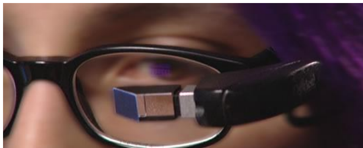
Fig. 2. An example of the MicroOptical head-up display mounted on eyeglasses.
