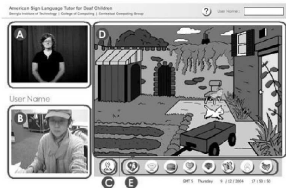
Figure 1. Screenshot of Game Interface. a) Tutor Video b) Live Camera Feed c) Attention Button d) Animated Character and Environment e) Action Buttons
