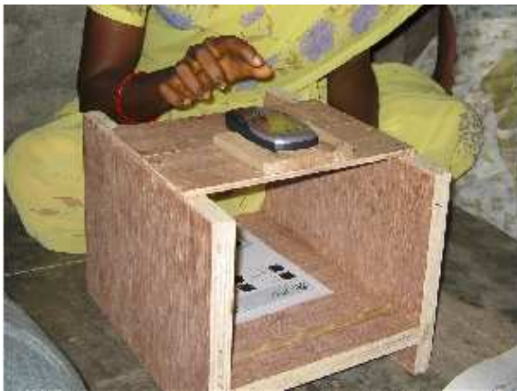
Figure 4. The BOX variation was a major improvement for users that had trouble with fine motor control. It fixed the paper document at the correct distance from the camera and stabilized the phone.
