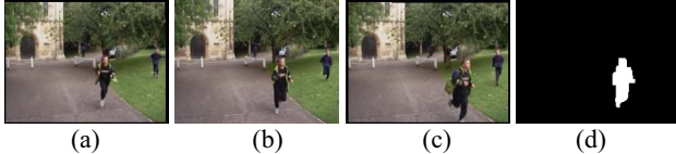
Figure 2. Scene motion detection: a) Previous frame warped to current b) Current frame c) Next frame warped to current d) Large moving area
